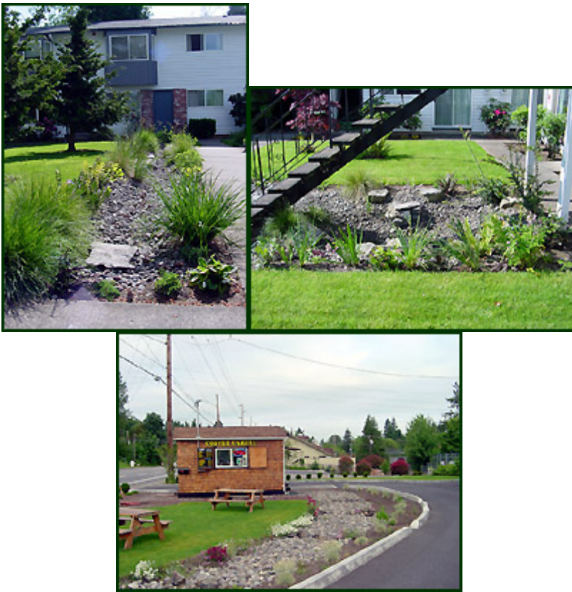
Examples of soakage trenches used in various areas including multi-family residential and circular driveway (Lower Columbia River Field Guide to Water Quality Friendly Development)
